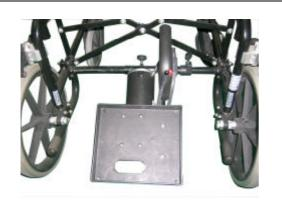
4. **Powerpack Installation.** Insert the spring loaded bar in to the bracket at the front of the powerpack. Install the spring-loaded bar with powerpack on to the 2 brackets now mounted to the wheelchair. Position the powerpack centrally and secure by tightening the 2 threaded knobs. Connect the powerpack to the handcontrol using the coiled cable from the powerpack.
