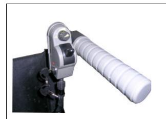
1. **Handcontrol Installation.** Unscrew the 2 short bolts from the back of the handcontrol using the allen key provided. Attach the handcontrol to the handgrip with the extra section by reattaching the 2 short bolts.
