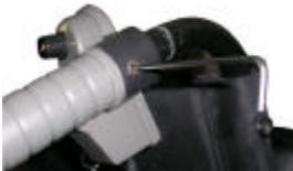
2. **Handgrip Installation.** Remove the existing wheelchair handgrips. Remove the rubber end from the PowerStroll handgrips and loosen the bolt inside the handgrip using the allen key provided. Slide the new handgrip on to the wheelchair push handle and retighten the bolt. Tighten up the 2 grub screws on the handgrip to secure the handgrip. Repeat for the other handgrip.
