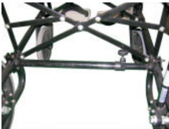
3. **Bracket Installation.** Unscrew both halves of the brackets and put together the 2 sections of the spring-loaded bar. Insert the halves of the brackets with protruding pegs in to the spring-loaded bar. Place the bar where it is required on the wheelchair (the spring in the bar will keep the brackets in position during installation). Attach the outer halves of the brackets using the threaded knobs provided. Remove the bar.
