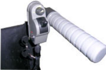
1. **Handcontrol Installation.** Unscrew the 2 short bolts from the back of the handcontrol using the allen key provided. Attach the handcontrol to the handgrip with the extra section by reattaching the 2 short bolts.
