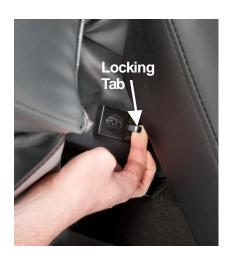
3. Pull on the backrest whilst pulling out the locking tab (arrowed) with your finger or a flat end screwdriver. This will release the backrest and allow removal.
