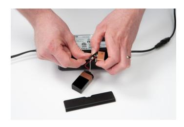
2. Pull out the two battery connectors from the compartment in the power supply and push a 9V battery on to each of the connectors.
