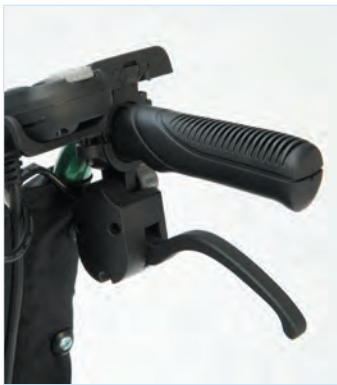
Hand control with variable speed dial, forward/reverse function, illuminated battery gauge and fingertip trigger control.
