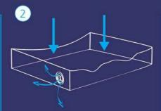
Apply pressure to the product and air is released through the pneumatic valve.
