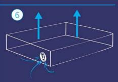
Once the pneumatic valve is re-opened air is drawn in and the cushion re-inflates to its original shape.
