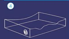
Once the pneumatic valve is closed the cushion retains its shape, even when the cushion is vacated.
