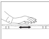
Test OneWaySlide's friction by rolling it and noting how easily it glides. Check to ensure that it resists movement in the opposite direction. If possible, compare with a new OneWaySlide.
